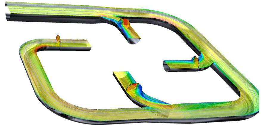
Flow distortion for a simplified Pelton 4 jet distributor
